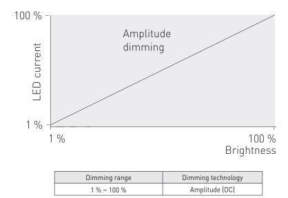
LC27MINI-FD-150-700 LED driver implements amplitude dimming technology across whole dimming range. Amplitude dimming offers the best available technology for dimming the light output in an accurate and flicker-free way to ensure high quality lighting in even the most demanding situations such as camera recording applications. Amplitude dimming technology complies with IEEE 1789-2015 recommendations of current modulation to mitigate health risks to viewers.
