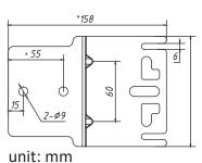
• Drill two holes in desired area and fix the luminaire firmly with M8 anchor bolts.
